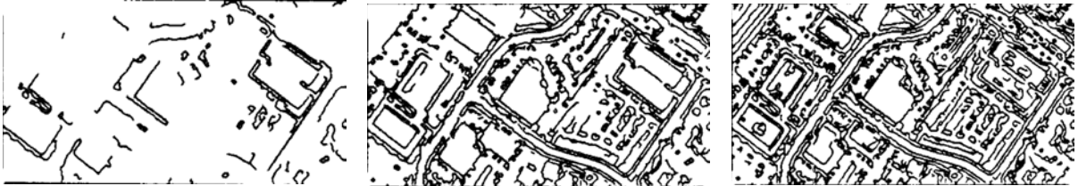
Figure 5. Canny edge images computed with progressively lower-edge strength thresholds (Canny, 1986)
