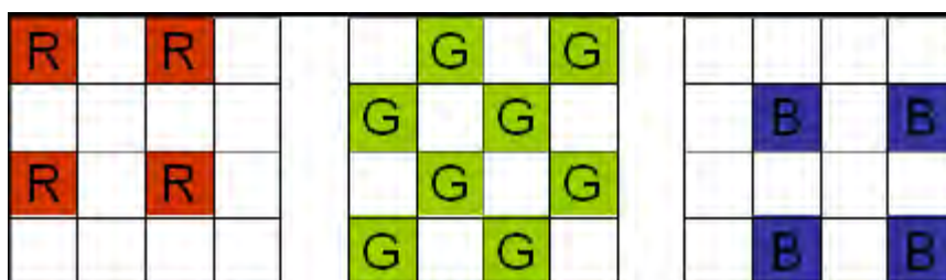
Figure 12. Bayer Sensor Decomposition (Guttosch, 2005)
